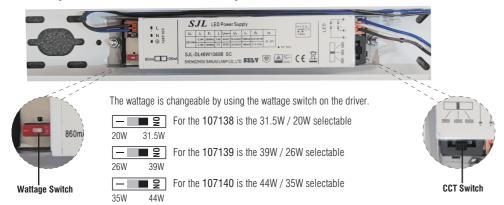
The colour is changeable between 3000/4000/6000K using the CCT switch on the driver before installation. Choose your preferred wattage and colour before installing by wattage switch or CCT switch on the driver. Note: Befeore you change the wattage or colour, please turn off the power switch for safety.
